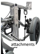
pic. 27: left front and rear attachment
