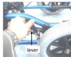
pic. 5: Activating the brake lever
