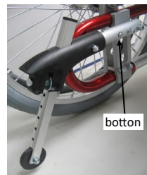
pic. 4.4: Detachable anti tip system
